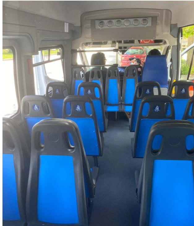
Construction of the passenger seats compliant with DM 01.04.2010 self-extinguishing, vandal-proof with abdominal seat belts, and handle.
