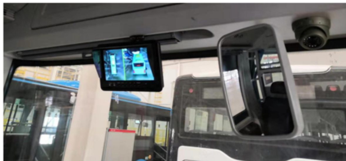
The in-vehicle monitoring and alarm is equipped with front and rear door monitors, and reversing radar.
